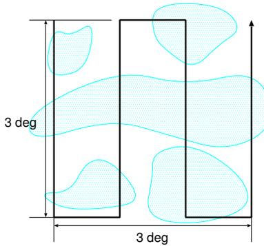
Figure 5: Alternative 3 AV-1 convective flight plan which maintains straight flight paths in the center of the pattern, but which would be better for highly disorganized convection.
