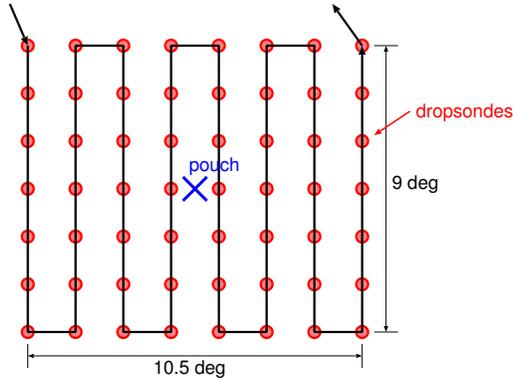
Figure 1: Broad flight pattern for AV-6. The 56 dropsondes (red circles) are spaced by  $1.5^\circ$ .
