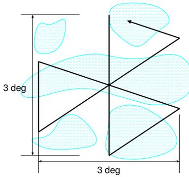
Figure 4: Alternative 2 AV-1 convective flight plan which maintains straight flight paths in the center of the pattern. Best for well organized, isolated convection.
