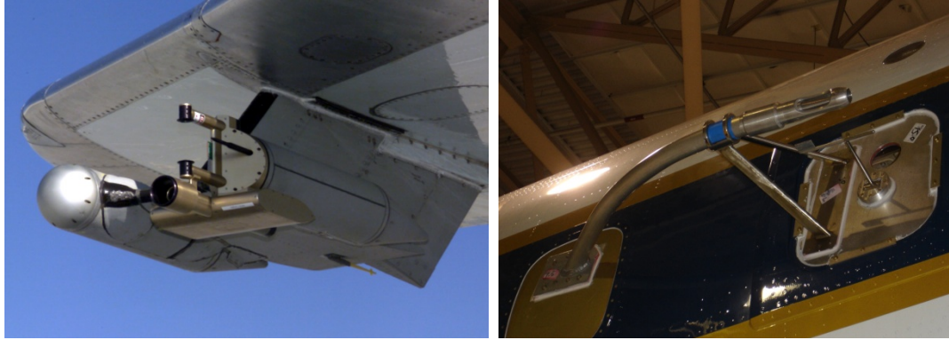
Figure 1. Wingtip-mounted Cloud Aerosol and Precipitation Spectrometer (CAPS, left) and the window-mounted iso-kinetic aerosol inlet (right) used to supply sample air to the LARGE instrument rack.
