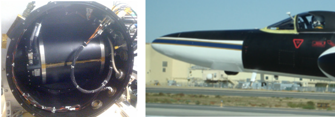
Figure 1. Left: Pressure vessel and cylindrical drum housing the AirMSPI camera. Right: AirMSPI installed in the nose of the ER-2 (visible protruding below the fuselage).
