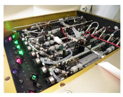
The combined AOP instrument package aerosol measures the properties necessary for calculations of radiative forcing and atmospheric heating rates. Further, the measured parameters can be directly compared to those derived from remote sensing measurements from satellite, airborne. and ground-based sensors. Additional measurements, such as the change in aerosol absorption and
