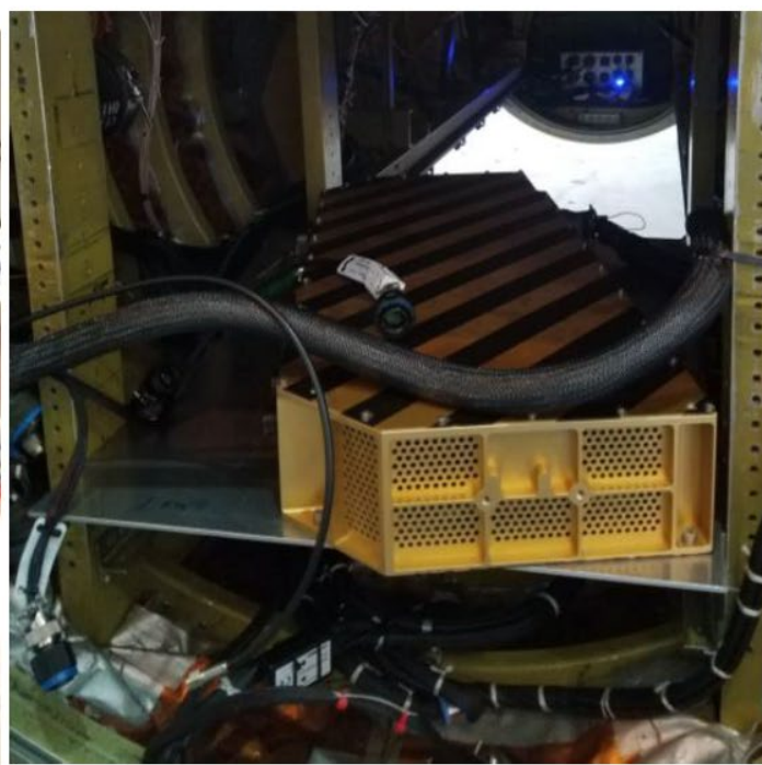
Figure 1.2: The Roscoe instrument in ER-2 configuration. On the left, the gold frame is the ER-2 interface rack, the orange insulated box houses the instrument, and mounted behind the box on the rack, is the laser power supply box. The data system is pictured in the photo to the right mounted to a plate in the midbody of the ER-2 superpod.
