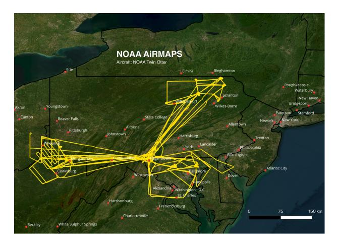
NOAA's Twin Otter aircraft flew over urban areas and coal shafts in Maryland, Pennsylvania, and the District of Columbia. Over the course of 20 days of flights, instruments including the Airborne Doppler Lidar, Picarro, TDLS, CES/CRDS, and PFP sampler gathered information about wind profiles and plumes of CO, CO<sub>2</sub>, CH<sub>4</sub>, H<sub>2</sub>O, N<sub>2</sub>O, and O<sub>3</sub>.
