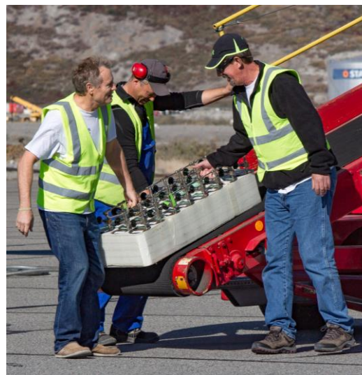
Exchanging WAS sampling canisters
