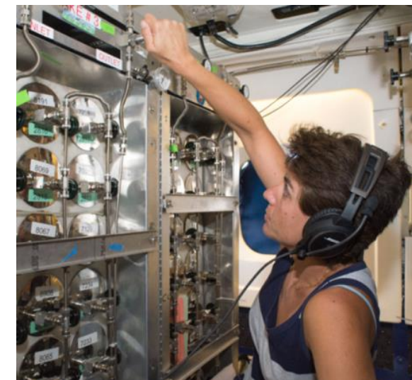
WAS sampling aboard the NASA DC-8
