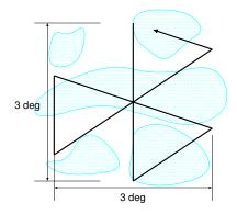
Figure 4: Alternative 2 AV-1 convective flight plan which maintains straight flight paths in the center of the pattern. Best for well organized, isolated convection.
