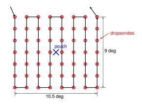
Figure 1: Broad flight pattern for AV-6. The 56 dropsondes (red circles) are spaced by 1.5°.
