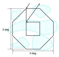
Figure 3: Alternative 1 pattern for AV-1 in which the HIWRAP Doppler radar is used to measure the wind field. The scale would change with the size of the targeted disturbance.
