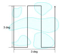
Figure 5: Alternative 3 AV-1 convective flight plan which maintains straight flight paths in the center of the pattern, but which would be better for highly disorganized convection.
