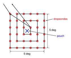
Figure 2: As in figure 2 except a focused pattern for AV-6. This pattern would be executed twice if possible resulting in  $2 \times 36 = 72$  dropsondes.
