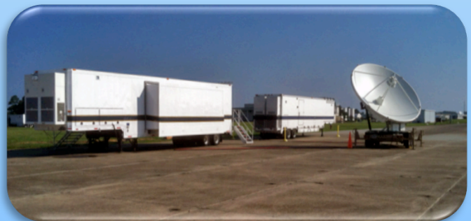
Global Hawk Mobile Operations Facility, Payload Mobile Operations Facility, and Ku Satellite Communications Dish
